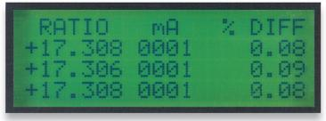
The ATRT-03B can also calculate the turns-ratio percentage error if the transformer's nameplate voltages are provided. The baseline turns-ratio is calculated using the nameplate voltages, and the test results are compared to the baseline turns-ratio. The percentage error is then calculated from the difference between the baseline and test turns-ratios.
